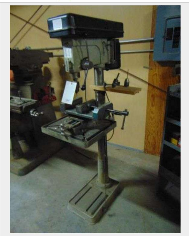
**Description**Model 951235. Powered by a 110VAC, 1HP motor. 3.75" stroke. Includes a Palmgren two axis vise, and extra chucks. Works.
